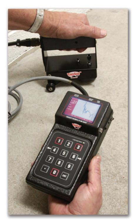
Measure the thickness of concrete slabs...
